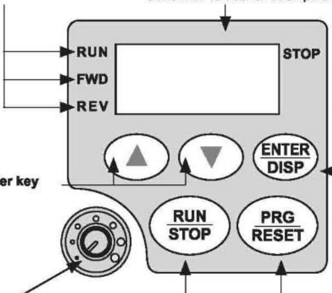
Turn to another frequency by rotating the potentiometer when the frequency is set to be controlled by the manipulator potentiometer
